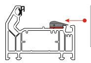
Fit a Frame Wedge "A" to include the packer "C" on the outer frame in the stay fixing area as shown
